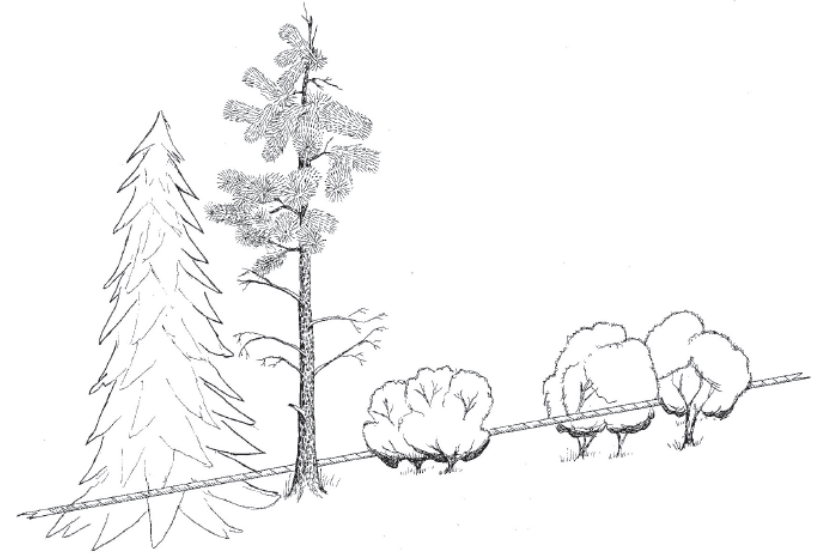
Figure LI-1 —The measuring tape is stretched taut below, in, or above the canopy vegetation, whichever position allows the easiest estimation of cover without the tape zigzagging around plants.
